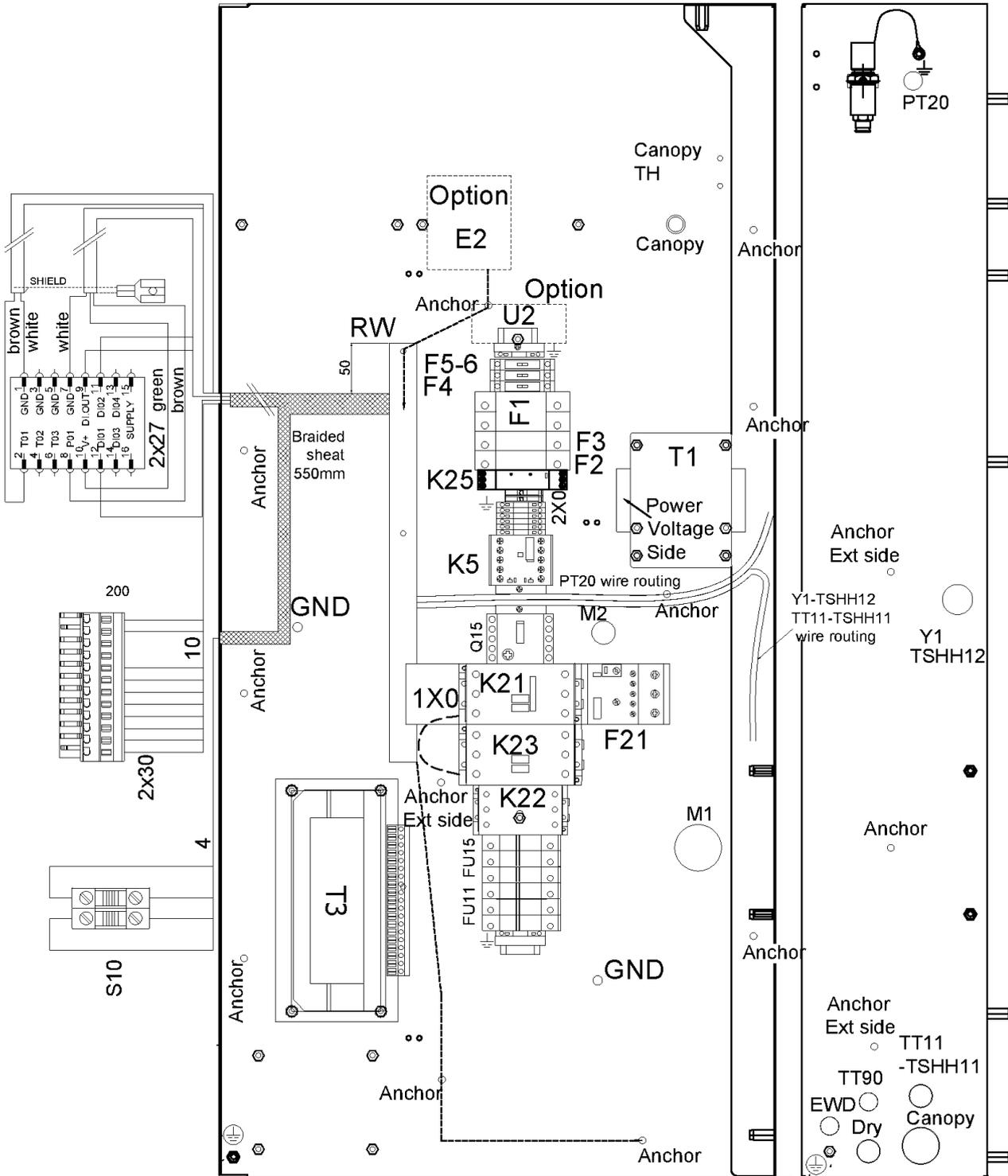
**43 - Cubicle components CPBg 20-34 - 575V/60Hz - Without dryer - Gear driven**
