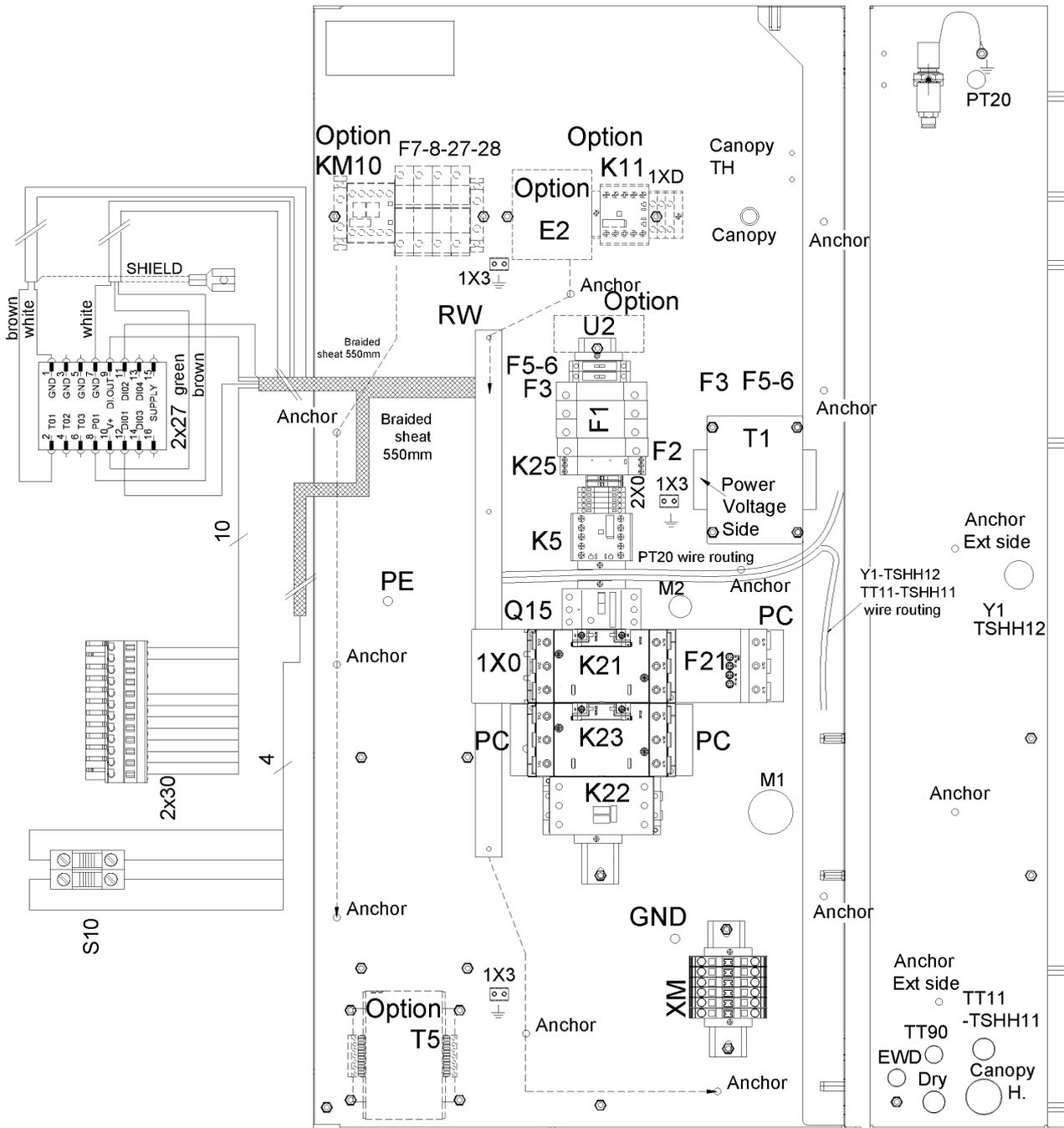
**37 - Cubicle components CPBg 20-34 - 230V/60Hz - Gear driven**
