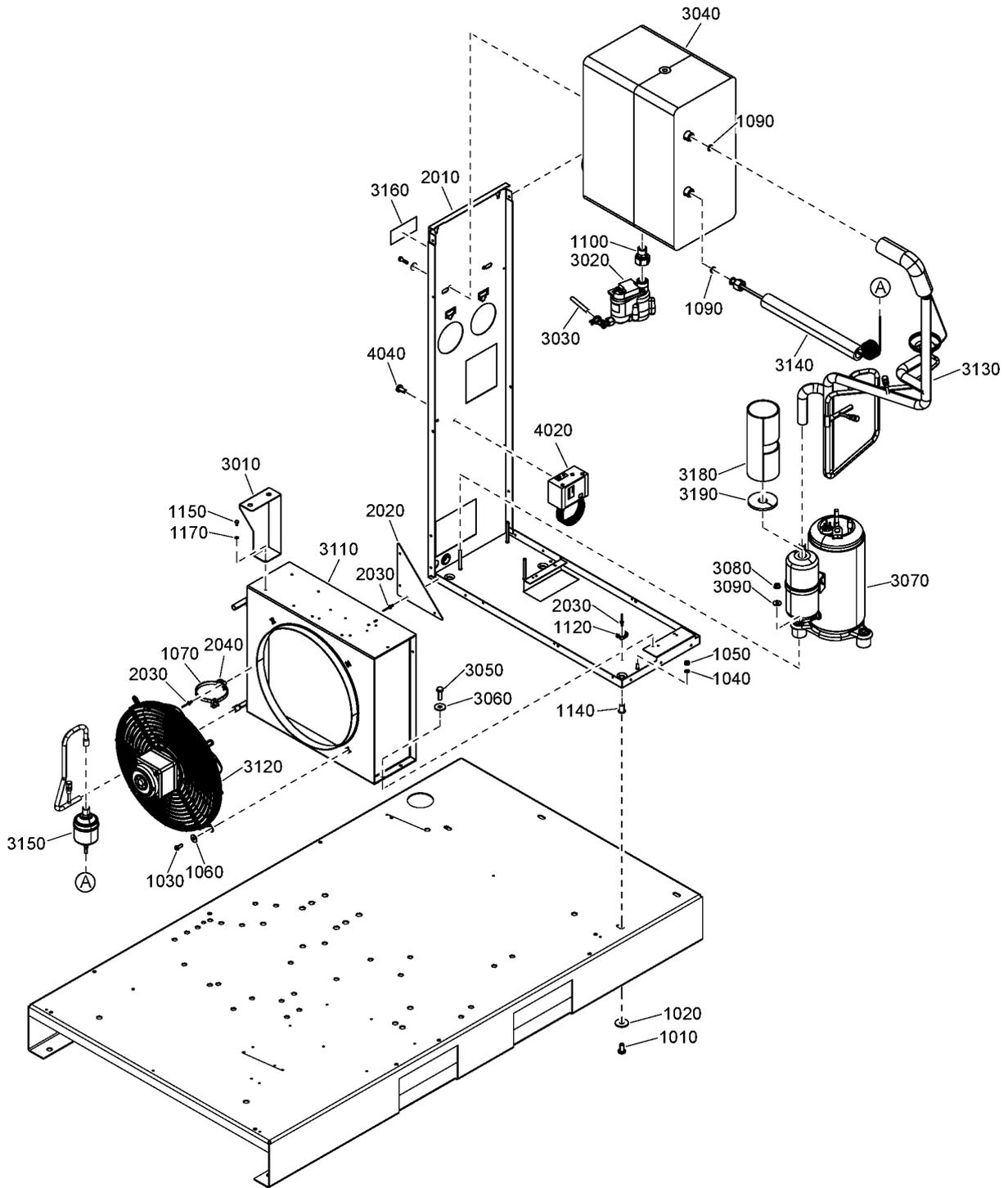
**31.10 - Components CPBg 25, CVPSd 25, CPBg 29, CPVSd 29, CPBg 34, CPVSd 34 - UL-cUL - 60Hz - ASME**
