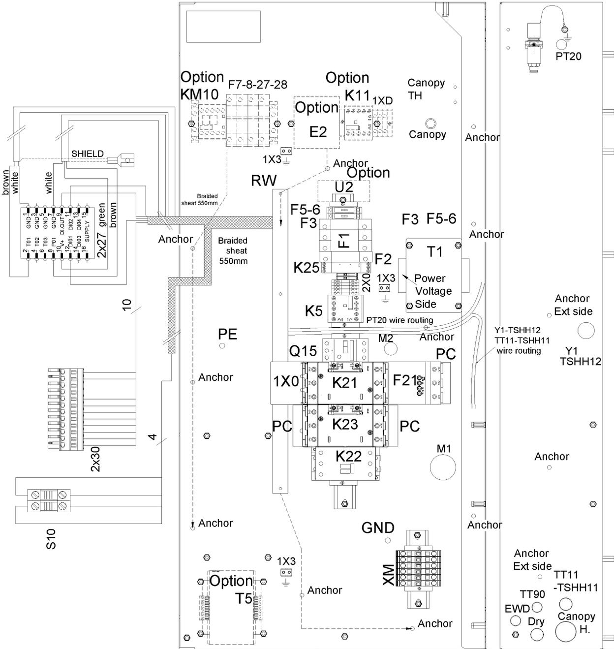
**36 - Cubicle components CPBg 20-34 - 230V/50Hz - Gear driven**
