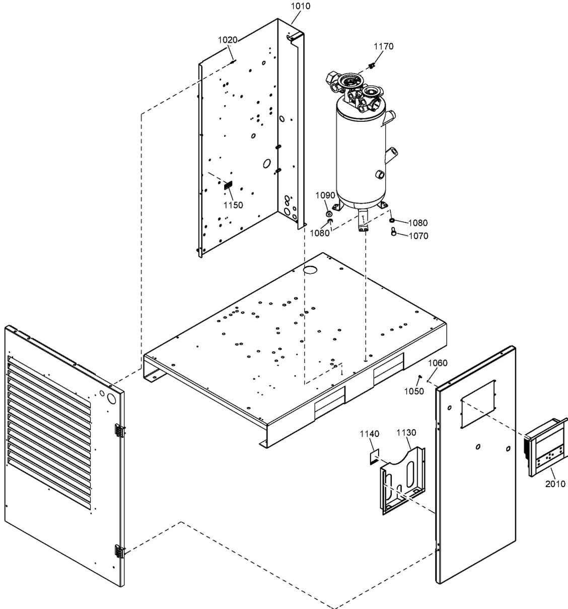
**32 - Regulation CPBg 20-34 - Gear driven – (AS1210, ASME, CE, MOM, SA – 400V), (CE – 230V), (ASME – 200230460V, 230V, 380V, 440V), (CRNASME – 575V), (CRNASME – 200230460V – With dryer)**
