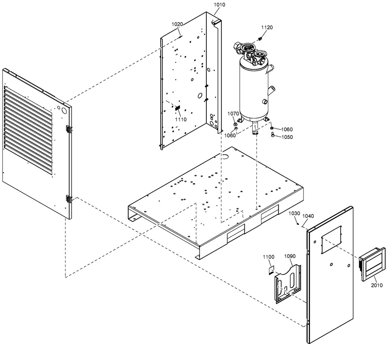
**33 - Regulation CPBg 20-34 - Gear driven - CRNASME - 200230460V - Without dryer**(MODEL:CPBG20\_18J , MODEL:CPBG25\_18J , MODEL:CPBG29\_18J , MODEL:CPBG34\_18J) + FREQ:60HZ + IDRY:N + MAPPR:CRNASME +
