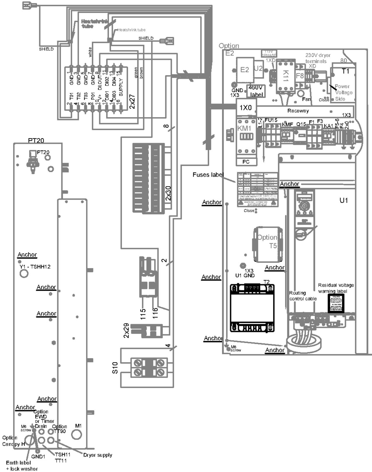
**49 - Cubicle components CPVSd 21-34 - 460V/60Hz - CRNASME - Without dryer - Direct driven**
