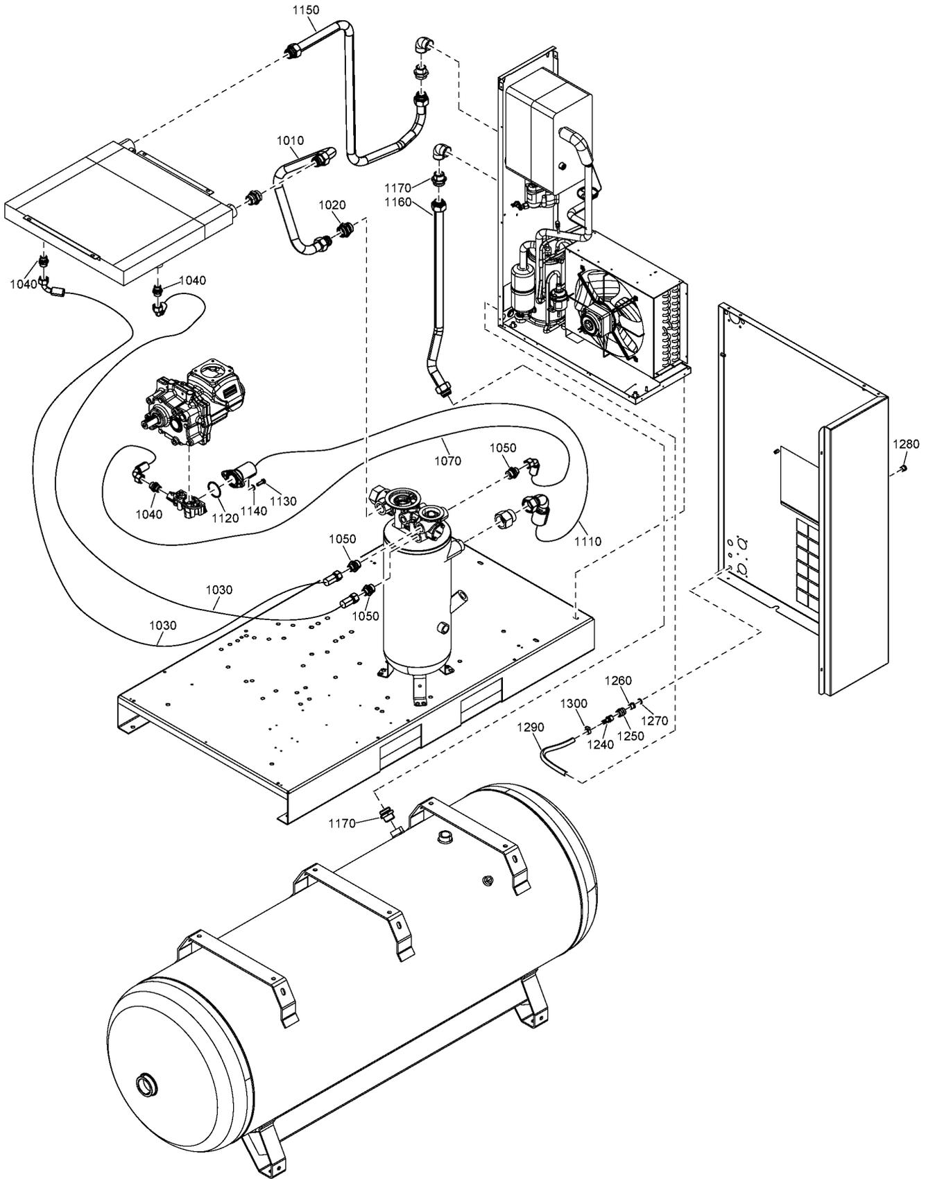
**23 - Air outlet CPBg 20, CPBg 25, CPVsd 21, CPVsd 25 - Tank-mounted - With dryer**
