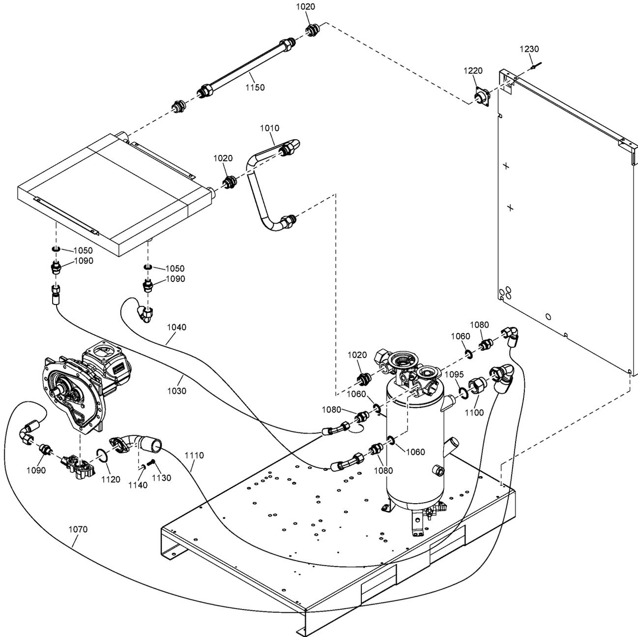
**16 - Air outlet CPBg 34, CPVSd 34 - Floor-mounted - Without dryer**
