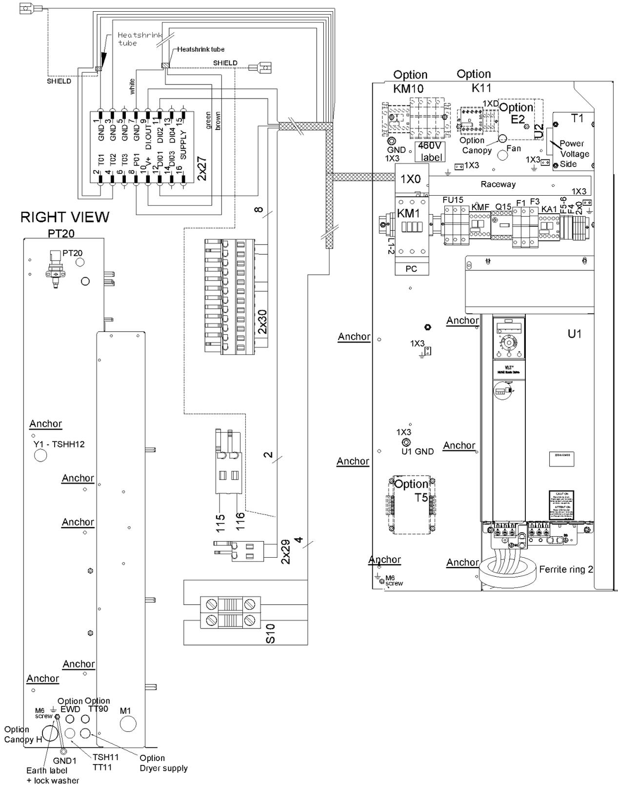
**48 - Cubicle components CPVSd 21-34 - 460V/60Hz - ASME, (CRNASME - Without dryer) - Direct driven**
