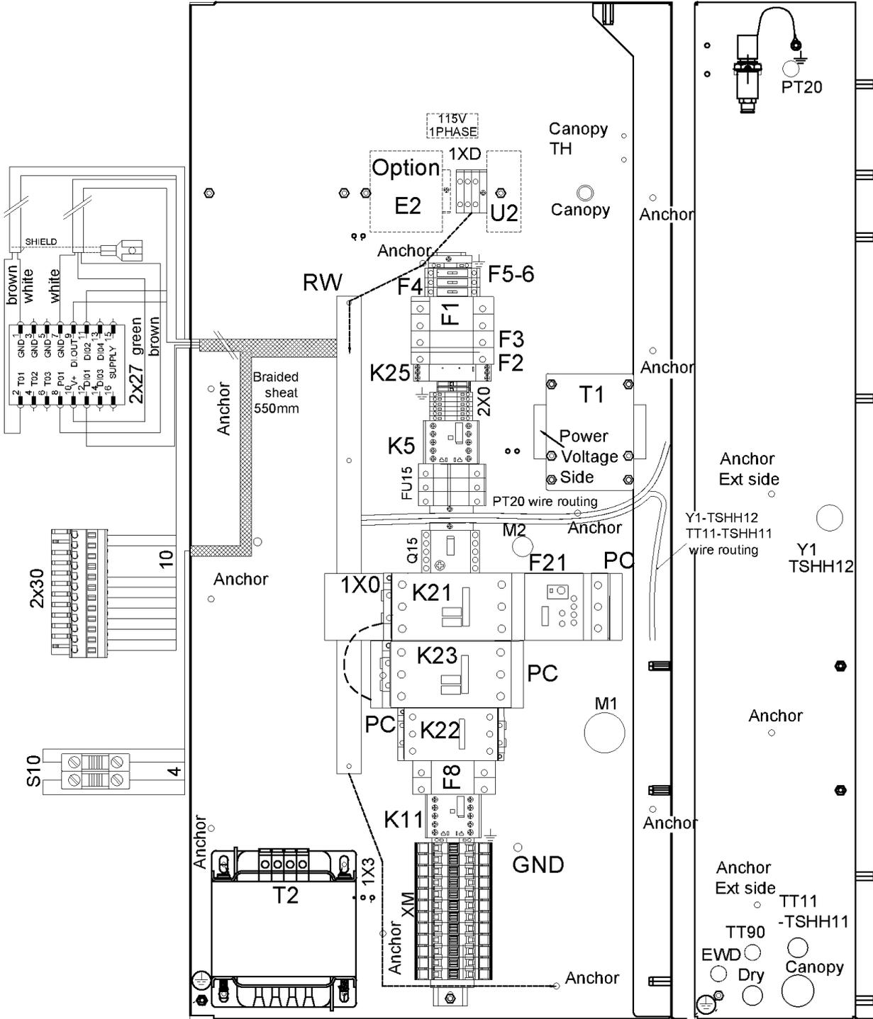
**40 - Cubicle components CPBg 20-34 - 200230460V - CRNASME - With dryer - Gear driven**
