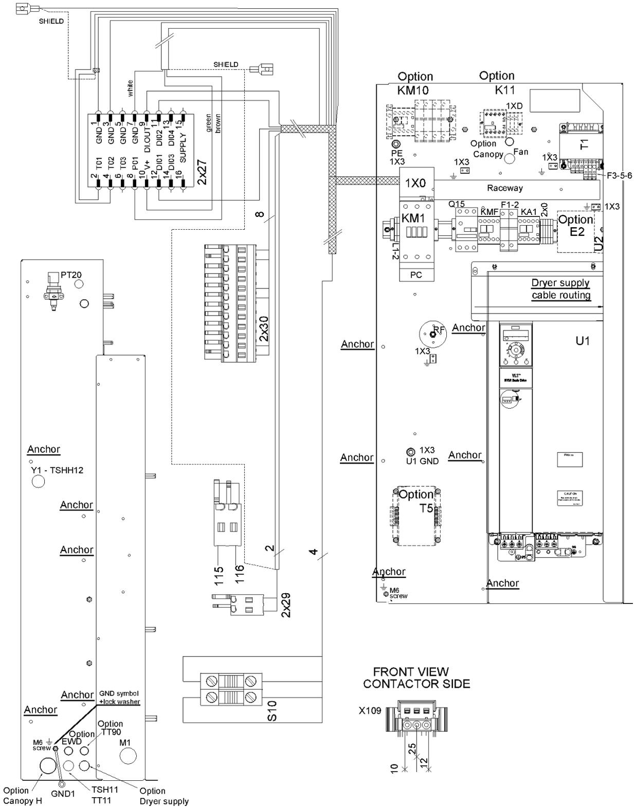
**45 - Cubicle components CPVSd 21-34 - 380V/60Hz - Direct driven**
