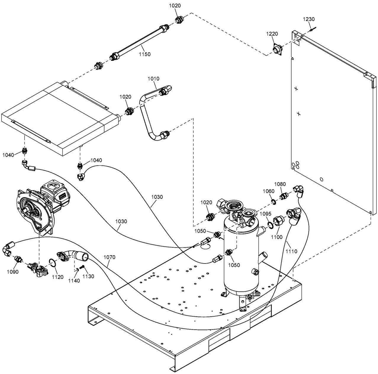
**15 - Air outlet CPBg 29, CPVSd 29 - Floor-mounted - Without dryer**
