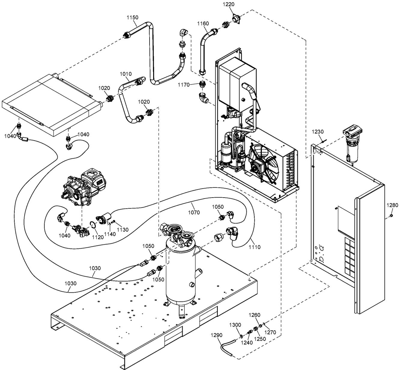
**20 - Air outlet CPBg 20, CPBg 25, CPVsd 20, CPVsd 25 - Floor-mounted - With dryer**
