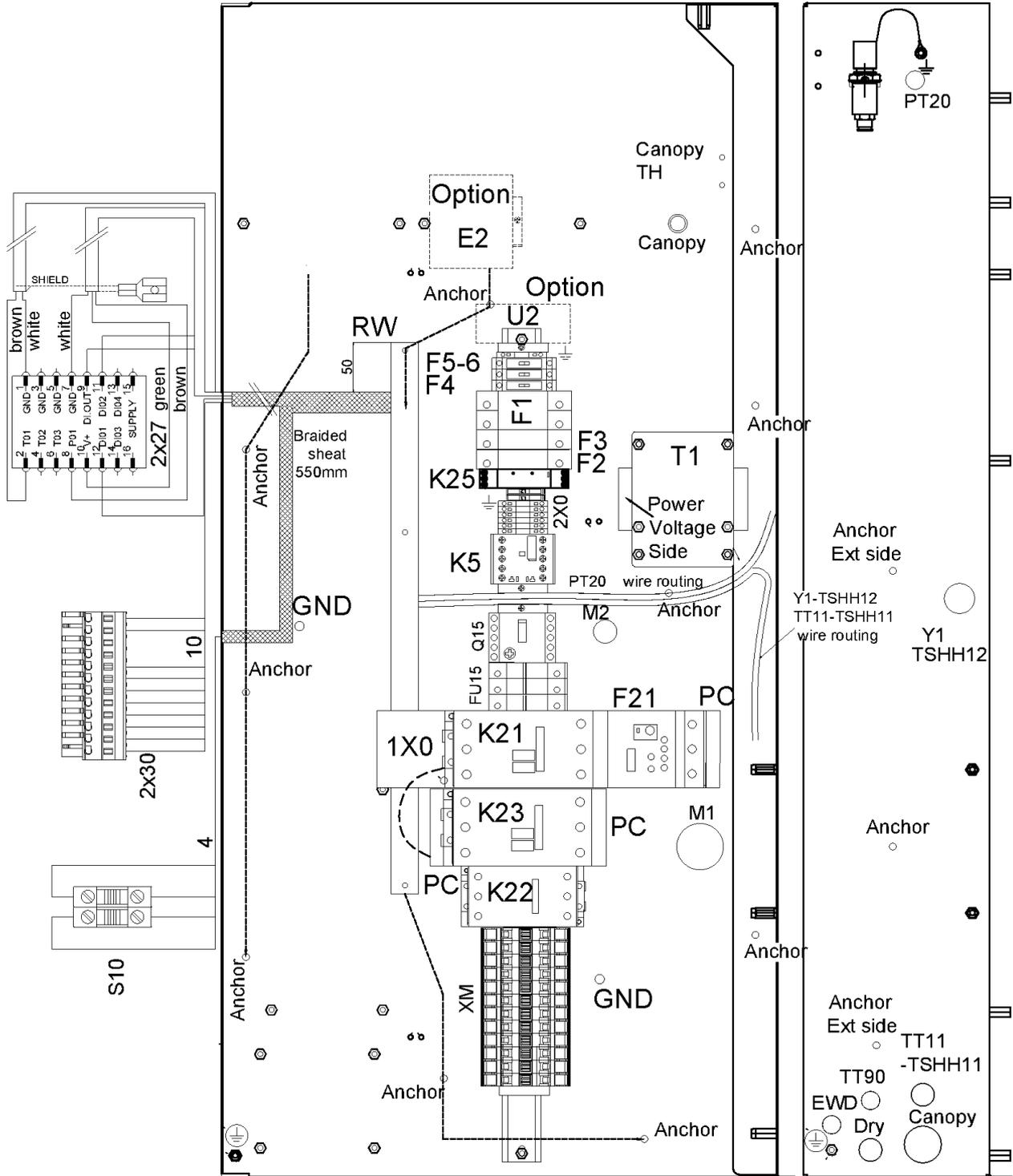
**39 - Cubicle components CPBg 20-34 - 200230460V - CRNASME - Without dryer - Gear driven**
