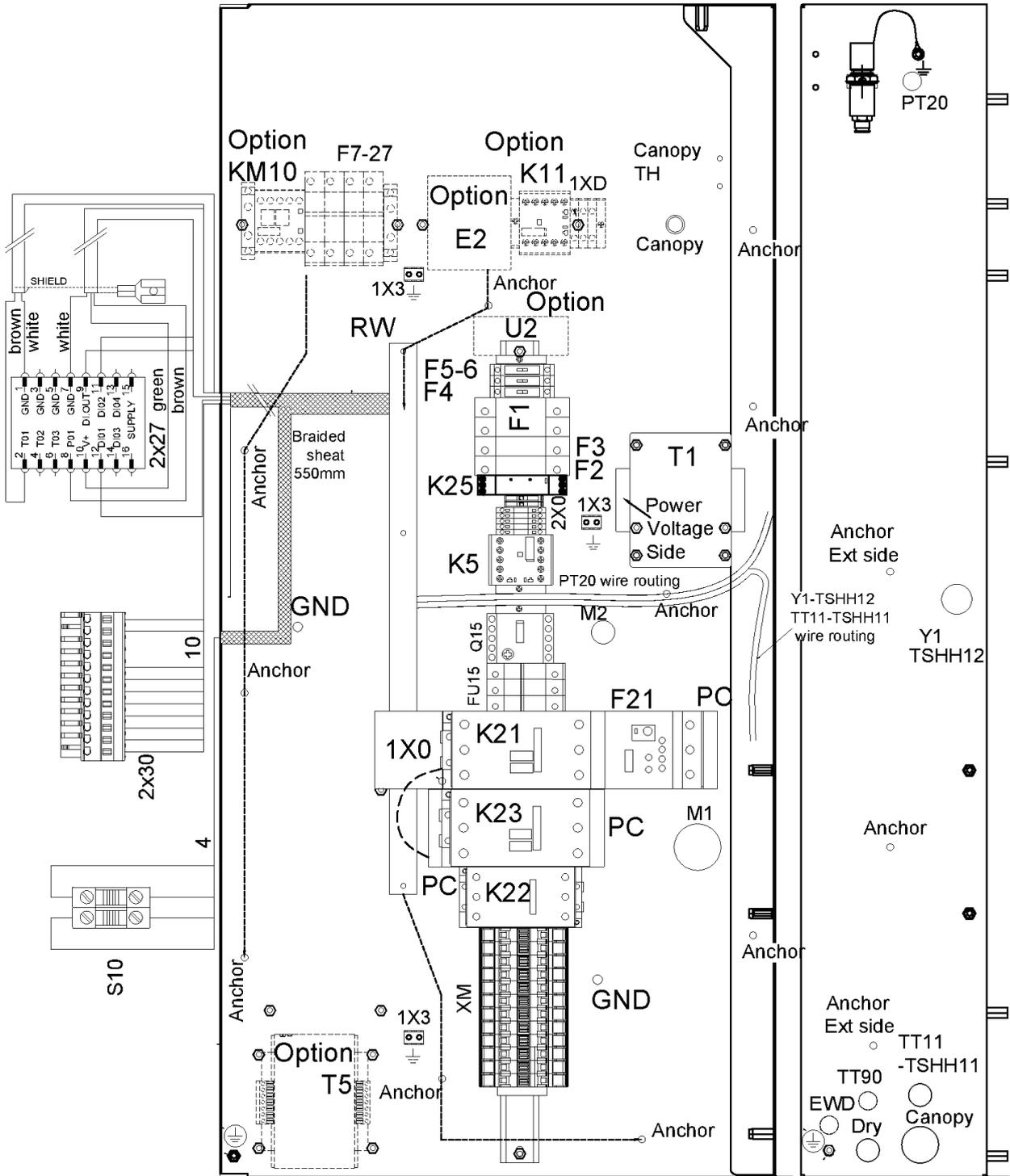
**38 - Cubicle components CPBg 20-34 - 200230460V/60Hz - ASME - Gear driven**
